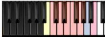
By pressing B-1 key (23) on the keyboard (the yellow key-switch), the instrument will randomise the sequence for as long as that key is pressed, generating new notes. When the key is released, the normal sequence will continue.
