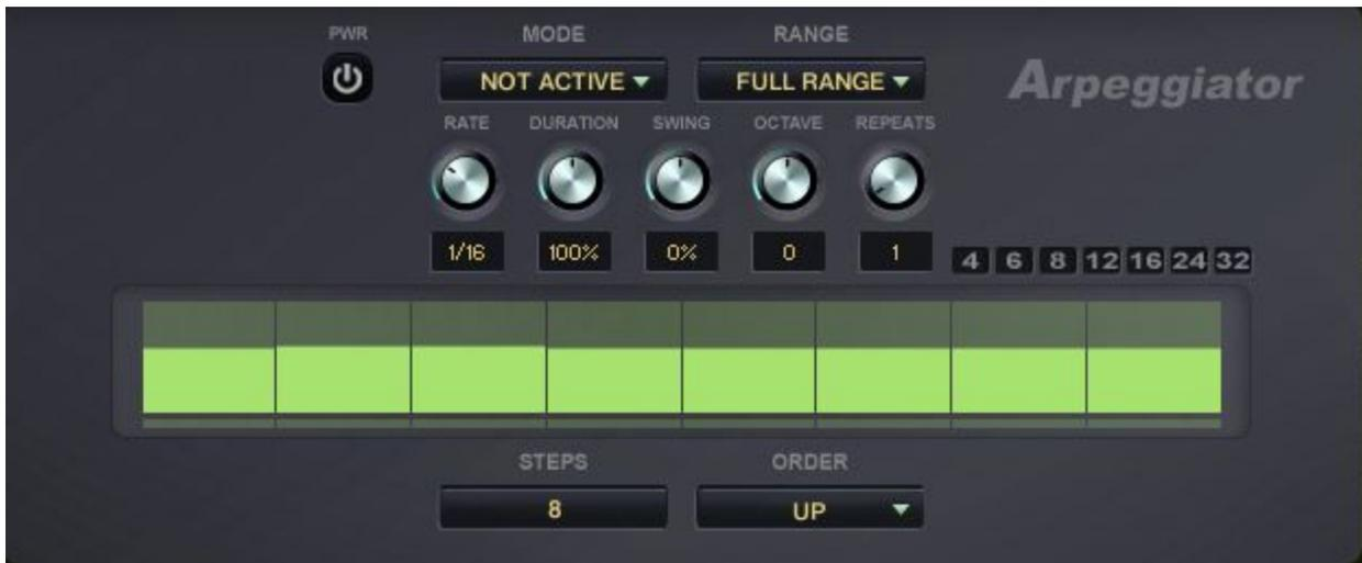
This new tool in Randomisers Series 1.2 is very powerful and can be used in conjunction with the step sequencers. By setting a slow rate ( $\frac{1}{4}$ ,  $\frac{1}{2}$ ,  $\frac{4}{4}$ ) the Arpeggiator can trigger each step sequencer, as the sequence will be triggered by the start of each arpeggiated note. Check the Starters Snapshots to hear the effect of both used in conjunction.
