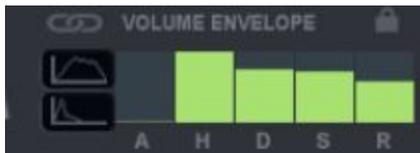
AHDSR CONTROLS: Attack, Hold, decay, Sustain and release per sound layer. When randomising a sound using the master randomisation buttons (Top of GUI) the state of these parameters will be maintained on the new sound allowing to generate new random sound which retain the volume envelope of the previous sound.
