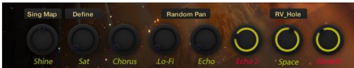
From version 1.1 the effect names act as effect bypass switches. On off state they cause the knobs to become all black, while they will retain the previous value. If the knobs amount is "0" the knob will appear all black even if the effect is not bypassed.
